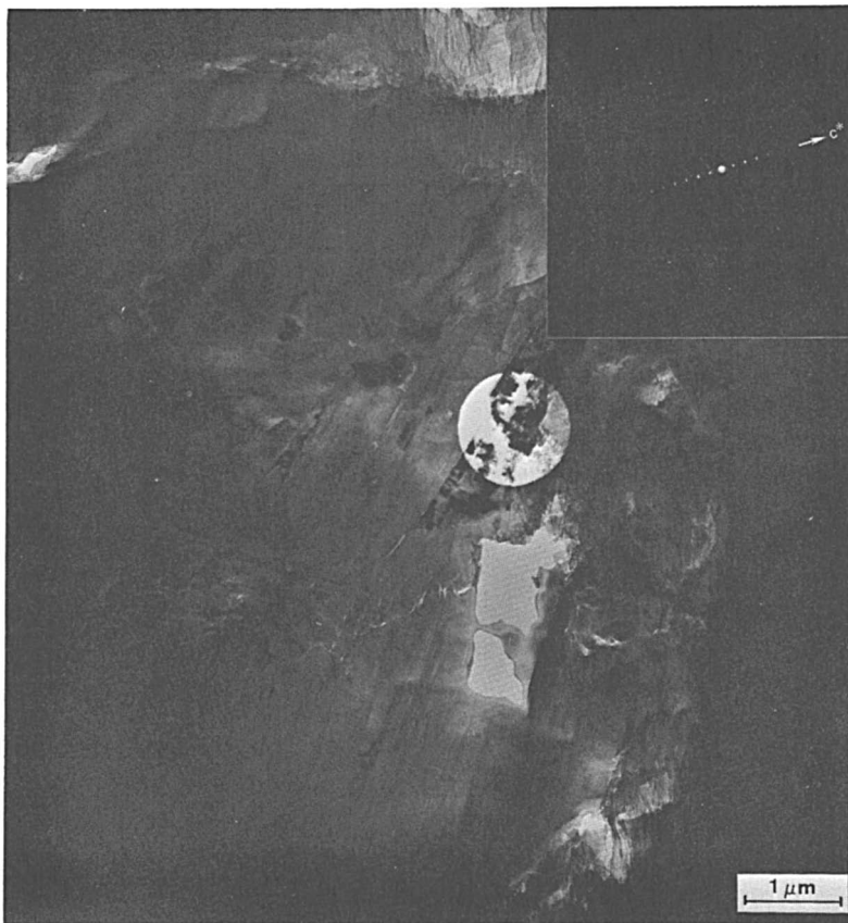
Figure 11. TEM micrograph of splint coal showing SAD pattern of kaolinite interbedded with vitrinite
