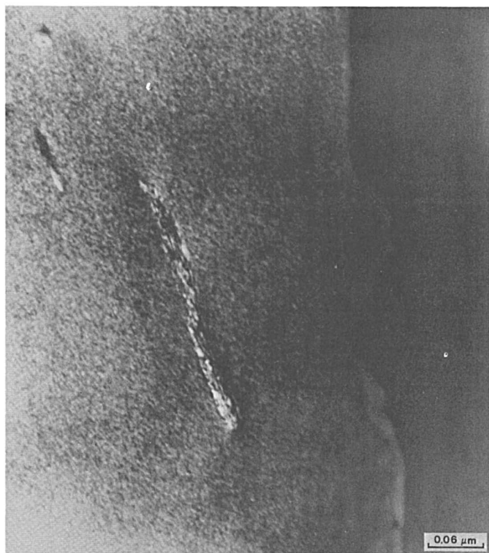
Figure 13. Dark-field, 0.36-nm ring image showing domains (bright spots)
