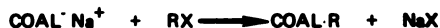
Figure 1. The chemistry of reductive alkylation involves two steps: one of reduction and one of alkylation. Our studies have utilized both sodium and potassium in the reduction step.
